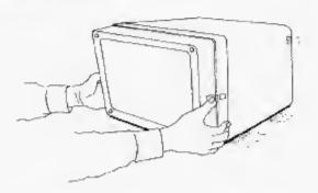
Carefully remove and set aside the cover. Then reach under the main part of the computer and pull out the keyboard. Be careful; the keyboard is permanently connected.
