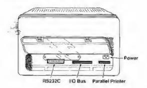
Connect the power cord to the power connector. Then plug the other end into the grounded, 120 VAC, 3-prong outlet. Because electrical interferences and surges can destroy data, do not use an outlet that powers other heavy equipment.
