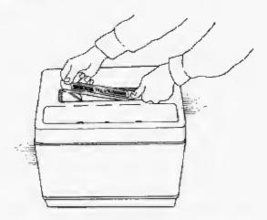
Set the computer where you'll be using it, near a grounded, 120 VAC, 3-prong outlet. Be sure the vents on the computer face up. Loosen the cover from the screen by pushing the latches back as shown here:
